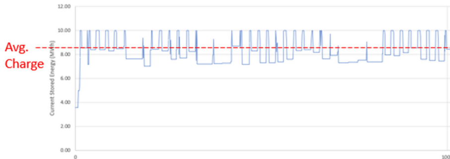
Figure 20: Sample of AMPeRRe Plotted Battery Charge for 8.7 MWh Reserve Charge
